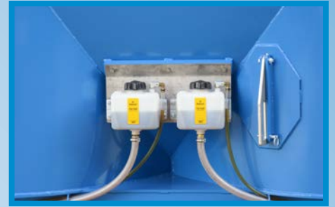
Gear oil expansion reservoirs are neatly tucked into the space between the two tubs.
