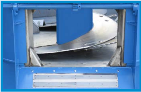
Discharge chute, magnet, and door frame are all stainless steel.
